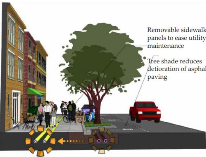
Figure 2: Move underground utilities under sidewalk, move trees into road bump outs
