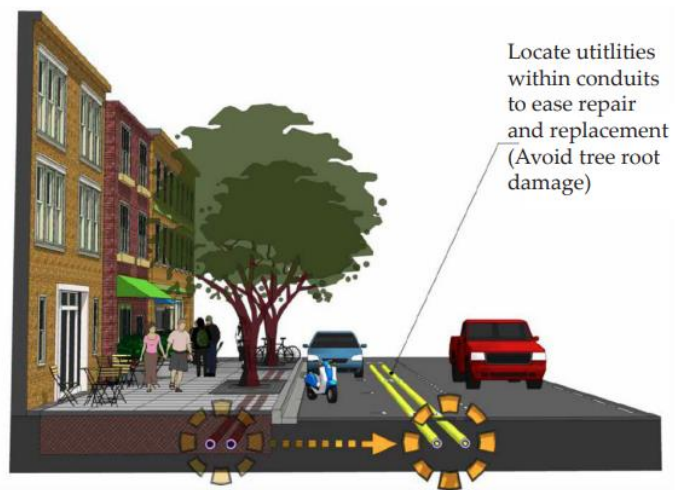
Figure 1: Move underground utilities under bike lanes
