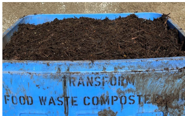
Figure 4. The one cubic meter insulated bin containing the blended food scraps/bulking agent mix.
