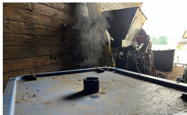
Figure 5. Photo showing the steam filled air rising from the passively aerated composting bin.
