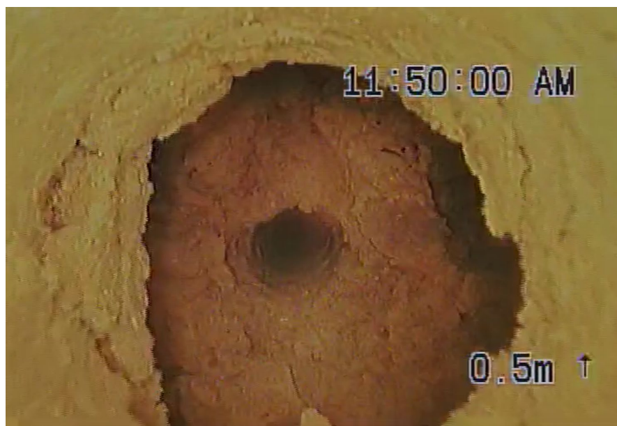
Figure 3: Screenshot of DCPT24-02 Void Taken from Downhole Camera Video Recording
